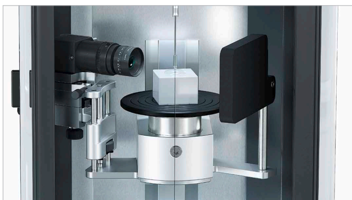
The optional camera records your adhesion measurement and paves the way for new methods.
